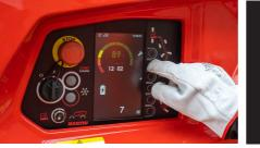
The large screen at the lower control box offers additional information to the top control box for operator and allows technicians to carry out a quick diagnosis, consult the machine memory and many
